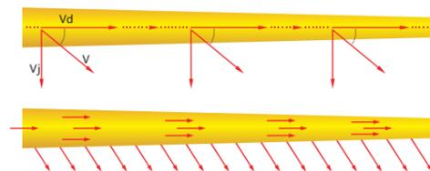
Uniform air velocity inside UR system results in same air dispersion direction along the duct.
