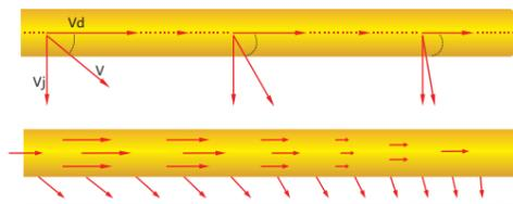
Due to vector superposition effect, there is wide difference in internal air velocity from inlet to endcap of ordinary equant round duct.
