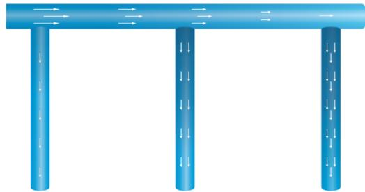
Different air velocity in main duct of Ordinary equant round fabric duct leads to different airflow supply in each branch, which causes the nearer the branch is to endcap, the more airflow the branch is to receive. ACD is required to balance airflow in each branch.
