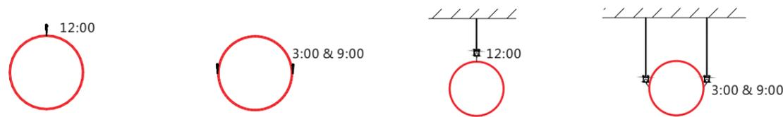
Single-row suspension system is applied to URR air dispersion system with tension cables installed at each endcap of straight runs so as to pull the duct surface round and taut and improve its aesthetic effect when the entire system is deflated.
