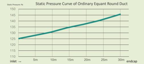
Since UR system is cone-shaped from inlet to endcap, its on-way resistance is larger than that of ordinary equant round duct. Meanwhile, the internal air velocity is relatively uniform and the static pressure regain is lower. The test result turns out that UR system could basically achieve balanced inner static pressure as long as it is not exceptionally long.
