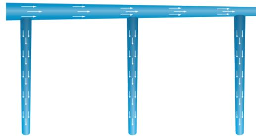
Since the air velocity in main duct of UR system is completely stable and balanced while the included angle between duct surface and branch duct is slightly less than 90°, that is conducive to lead uniform air distribution to each branch.
